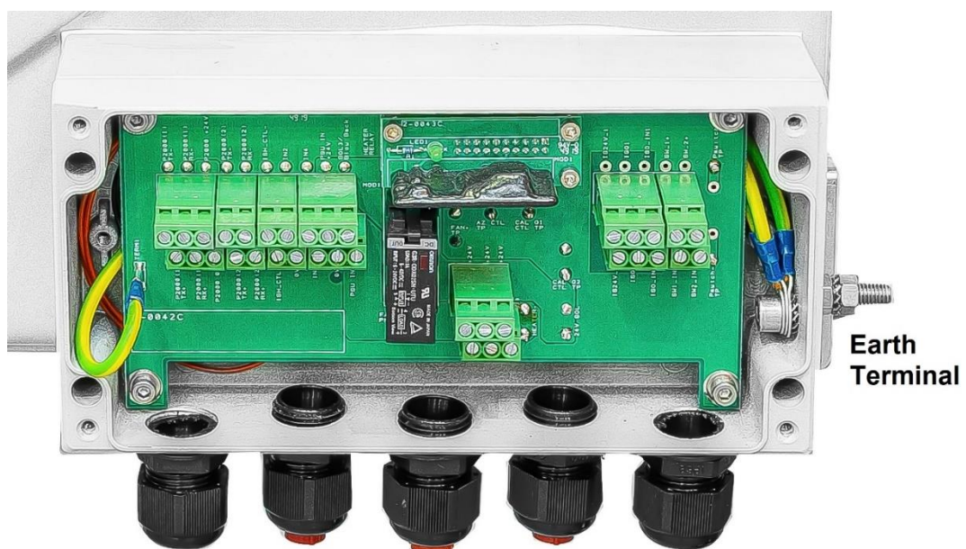
Figure 2-10 View inside P2000 Junction Box
